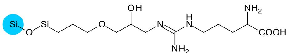
In HILIC mode, mainly acetonitrile/water mixtures are preliminary choice for mobile phase. High polarity elutes are strongly retained to ARG Silica by hydrophilic interaction. As water content increases, elution time is getting shorter. Thus, separation pattern of ARG Silica is different from RP mode that retention time is getting longer as water content increases.
